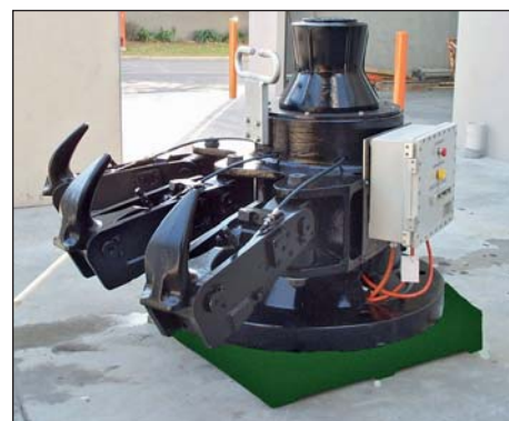
Triple 125T Quick Release Hook and Capstan Unit
