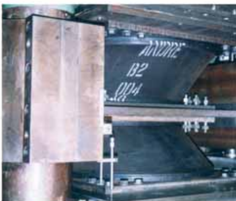
Andre High Damping Rubber Bearings under shear test on a 4000 ton bi-axial test machine.
