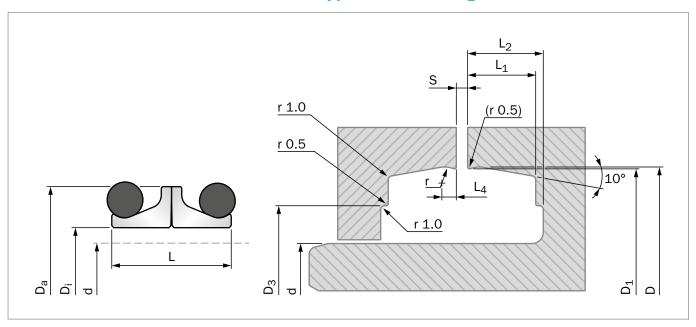
Figure 15: Installation Drawing
