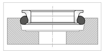
Figure 5: Correct installation of seal
