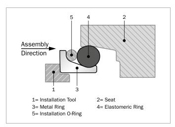
Figure 13: O-Ring as installation aid
