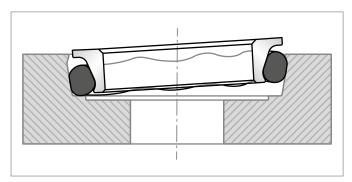
Figure 8: O-Ring slipped against the seat and waved against the metal ring
