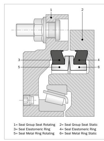
Figure 2: Mechanical Face Seals, Type DF
