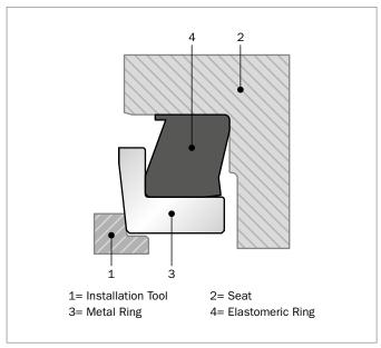
Figure 14: Installation Tool for DF Type
