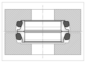
Figure 11: Upper half of the Mechanical Face Seal group has O-Ring slipped against the seat and on the seat bottom
