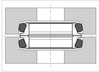
Figure 9: Correct seal assembly
