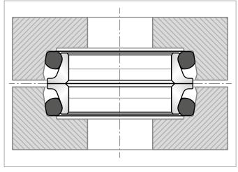
Figure 12: Both halves of the Mechanical Face Seal group have 0-Rings slipped against the seat and on the seat bottom
