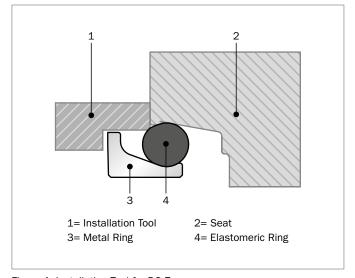
Figure 4: Installation Tool for DO Type
