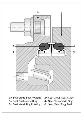
Figure 1: Mechanical Face Seals, Type DO
