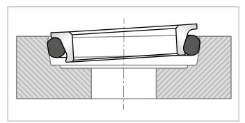
Figure 6: Metal ring slipped against the O-Ring
