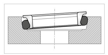
Figure 7: O-Ring slipped against the seat
