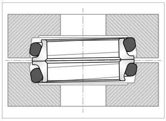
Figure 10: 0-Rings slipped against seats and Mechanical Face Seal group is tilted
