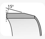
Inspect the spigot, socket and seal for damage and remove any dirt or dust prior to assembly. Chamfer the spigot end and remove all burrs.
