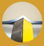
The support flange is retracted, and internal vacuum and external pressure forms the pipe around the contours of the seal
