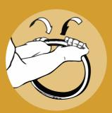
**Locate the bending zone of the seal**
