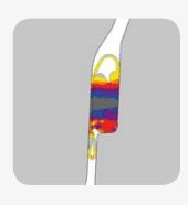
Lubrication of the socket or spigot is not required. Centre the joint and assemble. The position of the seal in the final mahole joint is shown.
