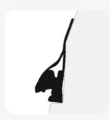
Stretch the seal onto the spigot and position against the shoulder.
