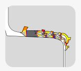
When the pipes or manhole sections are assembled, the rubber sealing element is designed to deform. This creates pressure on both spigot and socket, ensuring a watertight seal.
