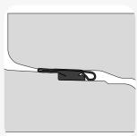
Center the joint and assemble. The position of the seal in the final joint is shown. If re-jointing is required ensure the sliding skin is drawn back to the original position.
