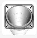
Equalize the stress in the seal by lifting and releasing at a few points. The seal must sit evenly against the spigot shoulder all around the manhole. Lubrication of the socket or spigot is not required.
