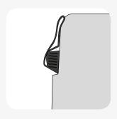
Stretch the seal onto the spigot and position against the shoulder.
