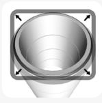
Equalize the stress in the seal by lifting and releasing at a few points. The seal must sit evenly against the spigot shoulder. Lubrication of the socket or spigot is not required.
