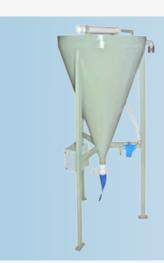
The Water Separation System recycles the water in a closed loop rather than requiring a continuous supply of fresh water. The System provides water, free of particulates. Typically, water from the system has a light milky white appearance. This water is suitable for coring and grinding machines.
