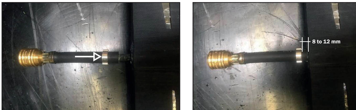
Figure 24: Mount the hose to the connection of the sealing bandage (left), position of the clamp (right)
