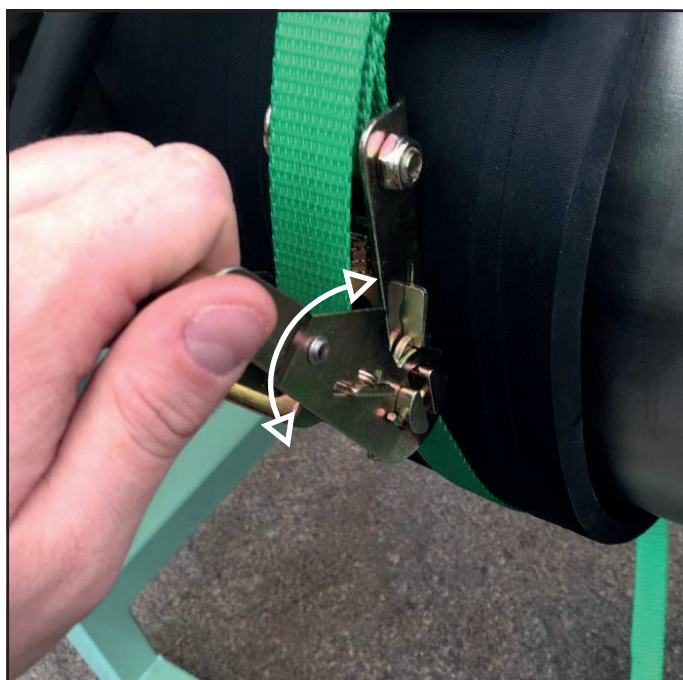
Figure 7: Tightening with the ratchet
