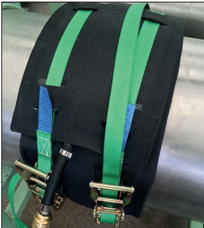
Figure 21: Mounted and inflated SAVA sealing bandage
