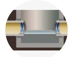
The compressive force providing the seal on either side of the joint is the result of increasing the effective diameter of the stainless steel expansion bands. The patented Slotted Band<sup>®</sup> is constructed from a single piece of 300 Series Stainless Steel precisely rolled to match the diameter of the CIPP liner.
