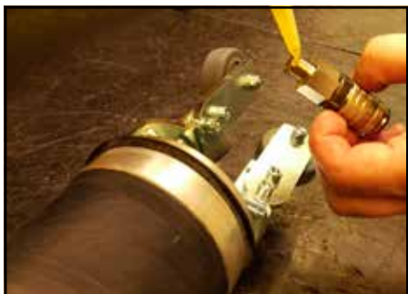
Figure 23: Application of Teflon adhesive tape
