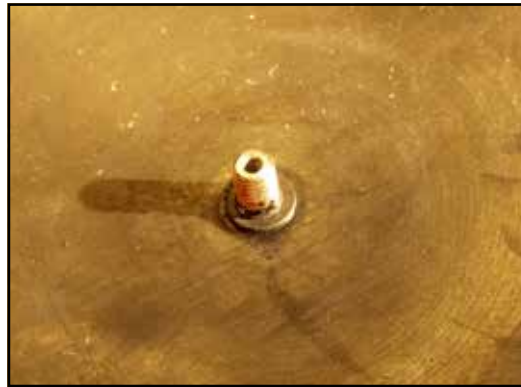
Figure 13: Screw the hat on the SAVA packer Figure 13: Threaded insert M6
