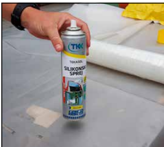
Figure 15: Apply silicone layer on the hat
