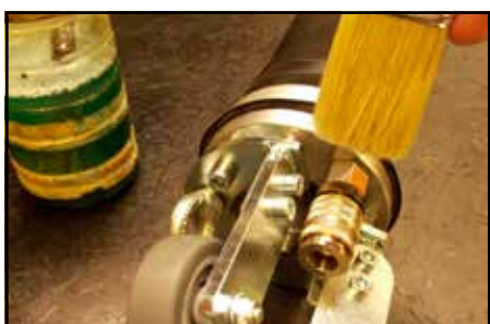
Figure 26: Check for leaks after replacing the connecting coupling
