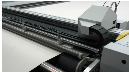
Hubergroup UK's CAD equipment provides a highly efficient means of producing small or large volumes of offset blankets from rolls.
