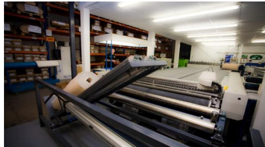
The CAD equipment at Hubergroup UK's plant is used to convert blankets from Trelleborg.
