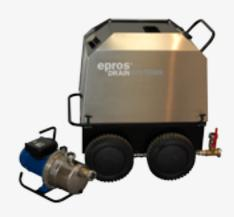
**epros®VacuumUnits,** by providing a constant and adjustable vacuum source, are key in the rapid and homogeneous impregnation of the liner felt – a crucial factor in complying with global quality standards set by engineers, specifiers, municipalities, authorities, industrial companies, etc.
