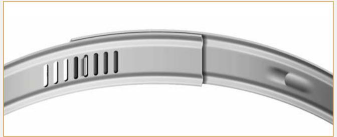
The band is then expanded using a hydraulic expansion tool. As the band expands the integral latching mechanism progresses from slot to slot, positively locking on each one until the next one is reached. There is an audible click created by the spring/rubber interaction as the band is expanded into place.
