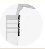
Install the top expansion band by collapsing it into itself and position it in the expansion band track of the rubber seal as shown at right
