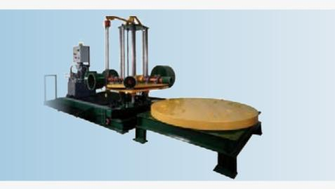
Hydrokor III is made for the large volume producer who needs to quickly and efficiently core drill several different hole sizes.
