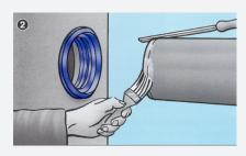
Chamfer the edge of the connecting pipe and lubricate it with Forsheda lub.
