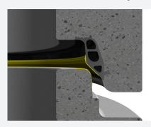
Centre the socket over the spigot and lower the upper manhole element to complete the joint. Light weight elements may require an additional vertical force to fully close the joint.
