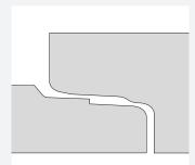
The wedge shaped design encourages self centering of the joint and is paticularly suitable for jacking pipe where a higher pressure robust joint is required. An 'S' version is available in a limited number of profiles with a reduced 'B' dimension where the design of joint or spigot length is not suitable for the standard seal. See 'Example of sizes' on page 2 for details.
