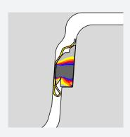
Lubricant has been applied between the sliding skin and the body of the seal. This design permits installation with very low force, as there is no friction between rubber and concrete. The special design of the joint and seal make the system easy to centre during jointing
