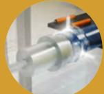
The pipe socket is cooled either by air or water and the mandrel withdrawn from the socket
