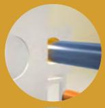
The pipe is heated to allow forming of the socket
