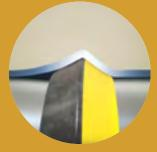
The support flange is retracted and internal vacuum and external pressure forms the pipe around the contours of the seal
