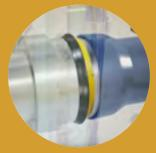
The mandrel is inserted into the softened pipe which flows over the seal thus forming the socket
