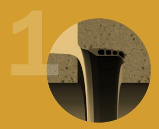
Check that the socket and spigot are in good condition and free from mud and gravel. Do not use damaged pipes. Apply lubricant to the spigot. This should be spread evenly over the entire surface paying special attention to the front radius of the spigot. Additional lubricant applied to the seal may further reduce the jointing force.
