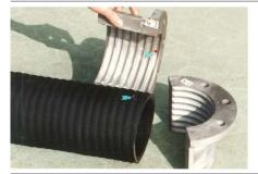
Position the half coupling N°2 on the hose in order to have the helix in the first corrugation: see green arrows.
