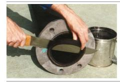
Cut off the hose with a knife standing on the face of the coupling (green arrow).
