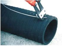
Curve the helix at 90° vs. hose axis then cut it with wire cutter or a hacksaw leaving 1 cm of the helix on the cover.
