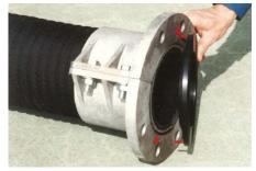
Put the gasket on the coupling putting the pin in the holes designed for that in the couplings (red arrows).
