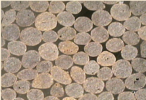
TESAEpoxy Ceramic Bead – 20x Magnification
