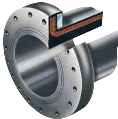
with a steel or stainless steel backing ring for medium working pressures. The Double Action® flange; a form-fit flange construction for higher working pressures, and suitable for very high axial loads. Vulcanized flange couplings for every working pressure, with optional swivel flanges, in accordance with the DIN and ANSI norms, for easy fitting.
