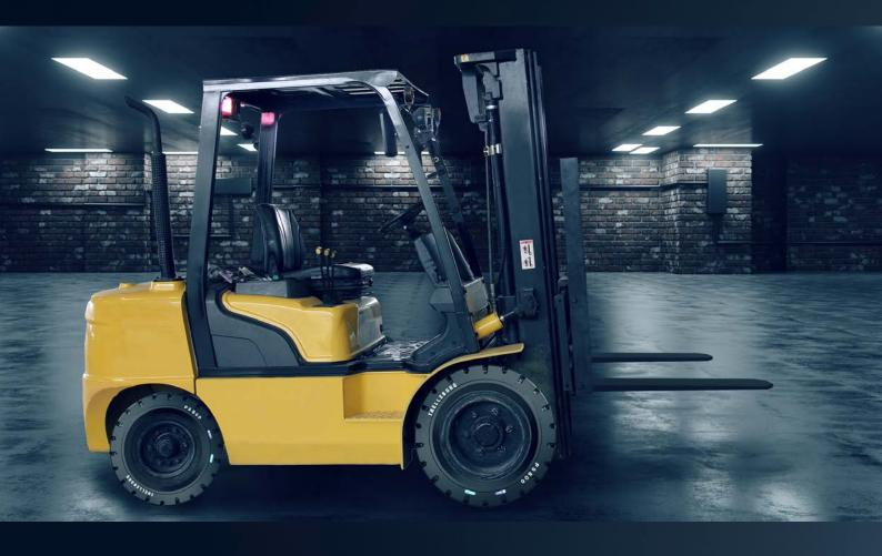
The Trelleborg PS800 is the newest press on solid tire for medium intensity applications, versatile in all working conditions.
