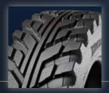
The progressive widening of lugs towards the shoulder, and the distinctive terraces design, increase self-cleaning and traction.
